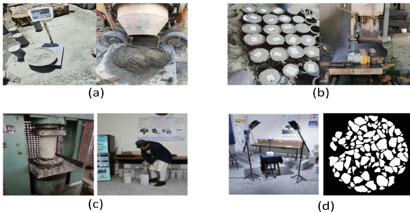
Fig. 2. Experimental workflow: (a) casting, (b) curing and cutting, (c) Testing, and (d) imaging of specimens.
