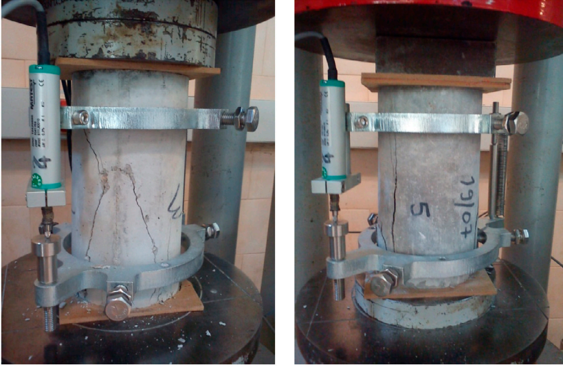
Figure 3. Uniaxial compression test set-up.
