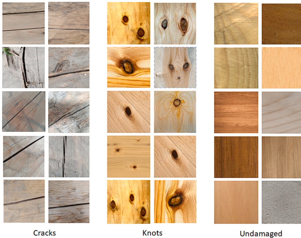
Fig. 4. Example images for each of the three subsets of the dataset: (i) Cracks; (ii) Knots; and (iii) Undamaged.
