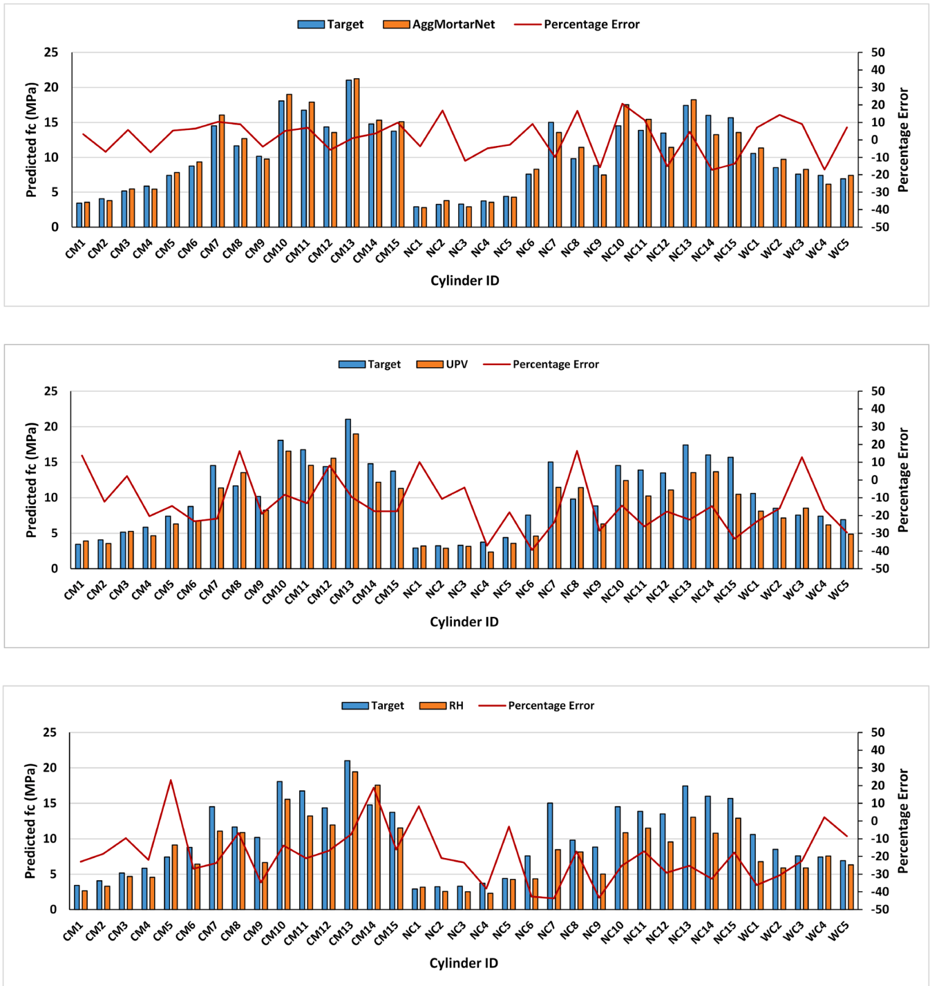
Fig. 21. Comparison of percentage error in concrete compressive strength predicted by ANN (top), UPV (middle), and RH (bottom).
