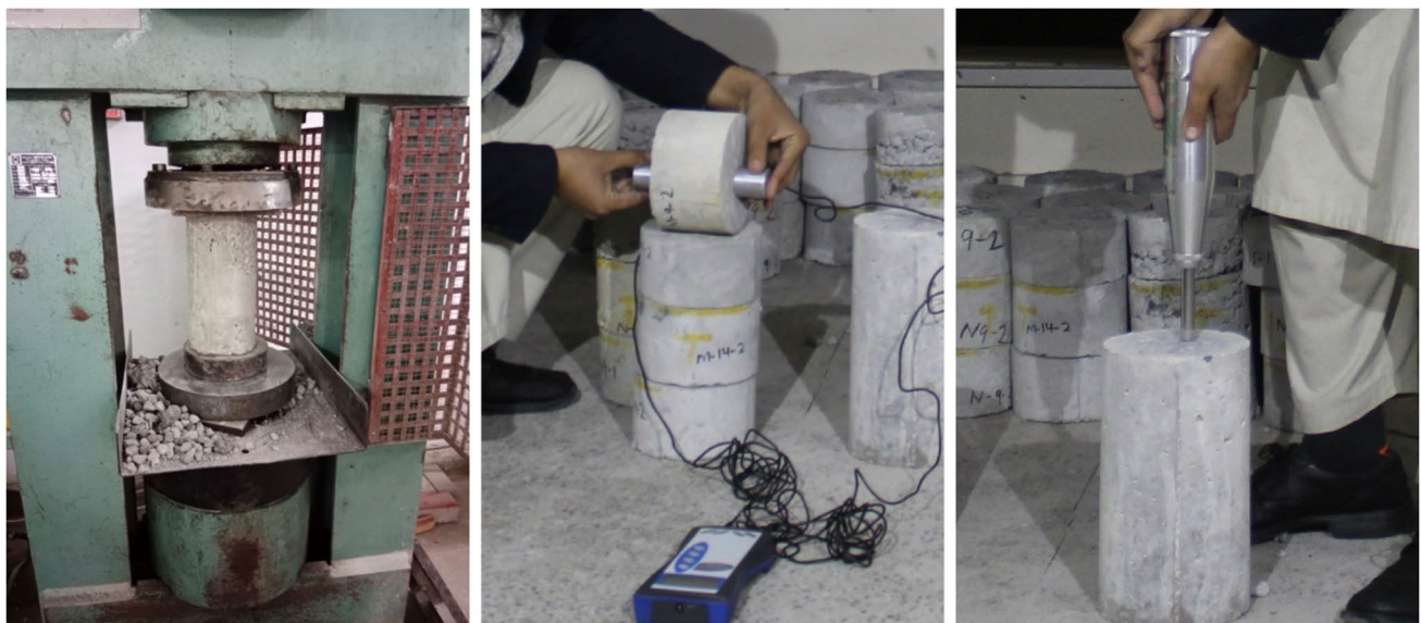
Fig. 13 Testing setup for assessing mechanical properties of concrete; Compressive strength test using a universal testing machine (left), Ultrasonic pulse velocity (middle), Rebound hammer test (right)
